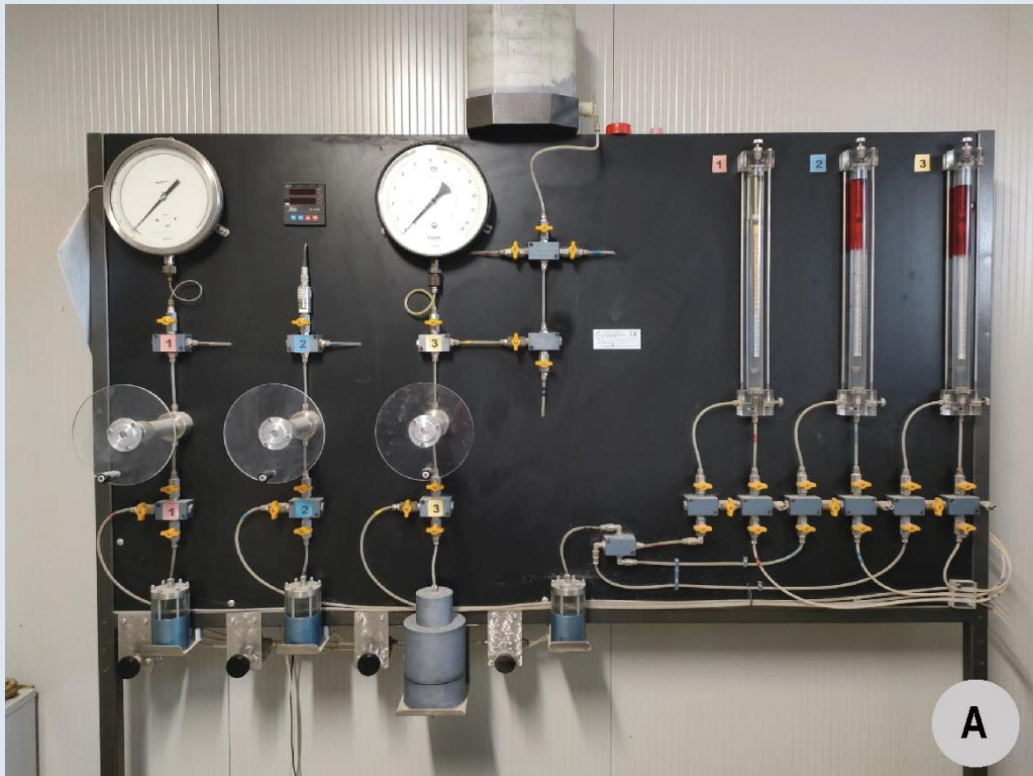
TRIAXIAL TEST APPARATUS: A) Control panel B) Triaxial cells
